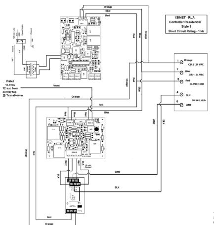
Connect supply valve to pins 4 & 5.
